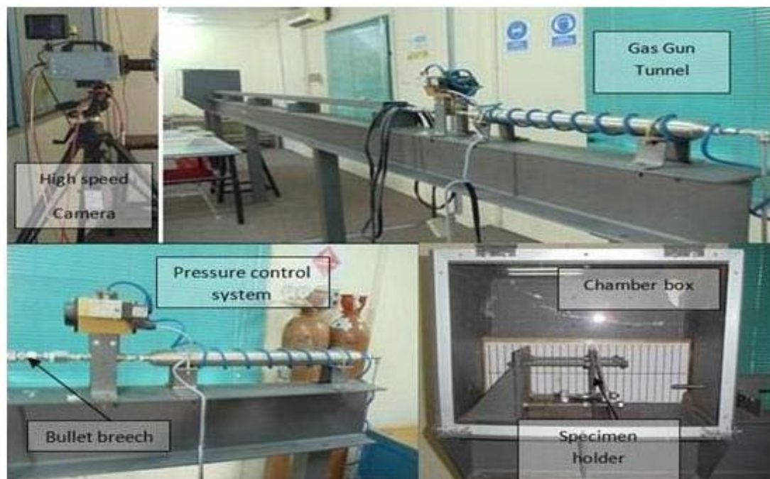
Figure 7: Gas gun tunnel for conducting the ballistic impact test.
